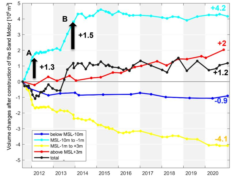
Figure 3.19 Volume changes within the Delfland coastal cell since 2011
