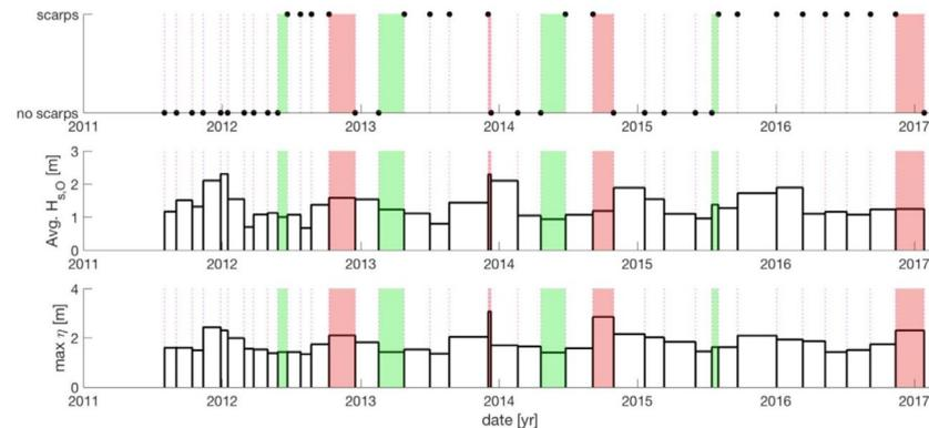
Figure 3.10 Occurrence of cliffs on the Sand Motor in relation to the average wave height ( $H_{s,0}$ ) and wave run-up height ( $\eta$ ). Green : developing cliffs; Red : erosion of cliffs (De Schipper et al., 2017; Van Bemmelen et al., 2020).
