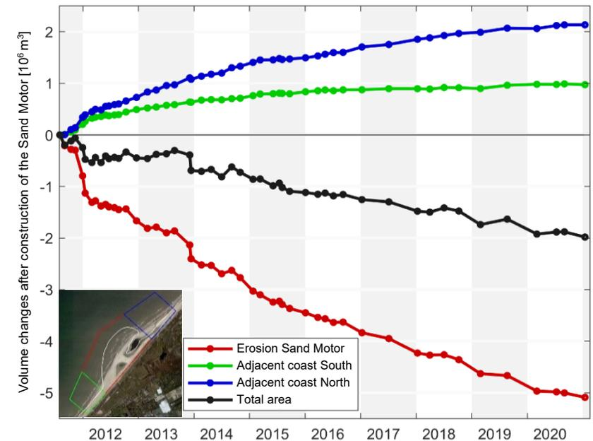
Figure 3.18 Changes in the measured volume of sediment in the first 10 year after construction of the Sand Motor (Huisman et al., 2021).
