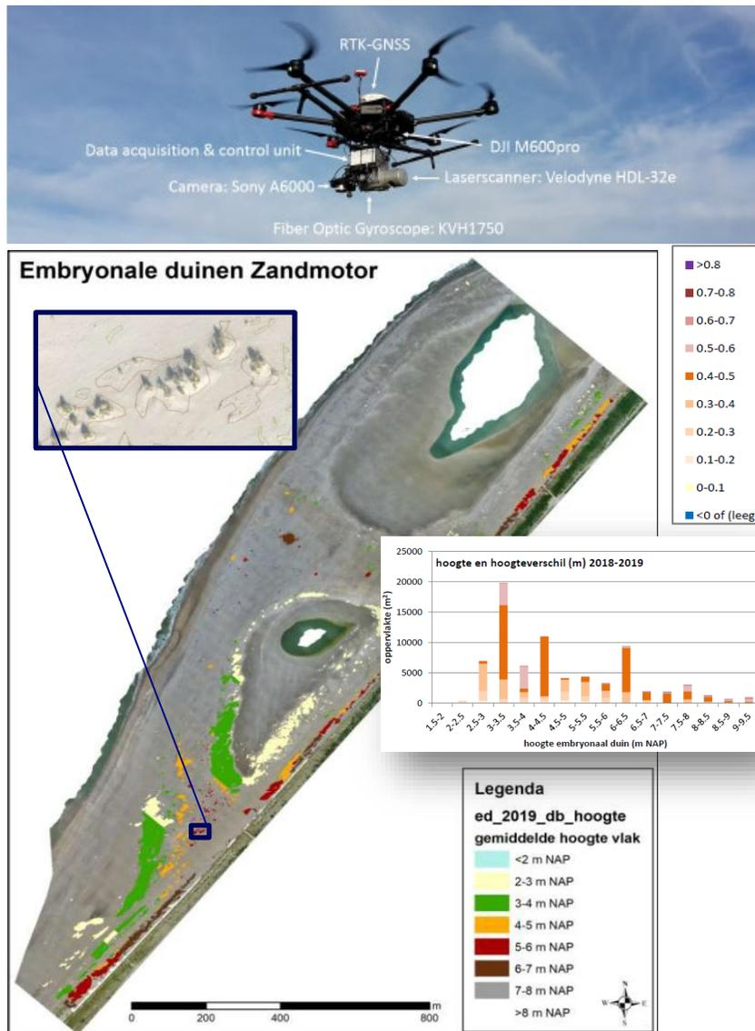
Figure 6.1 Monitoring of the height of embryonal dunes with a drone (Upper: Shore, 2020; Lower: Arens, 2021; Huisman & the Vet, 2021)
