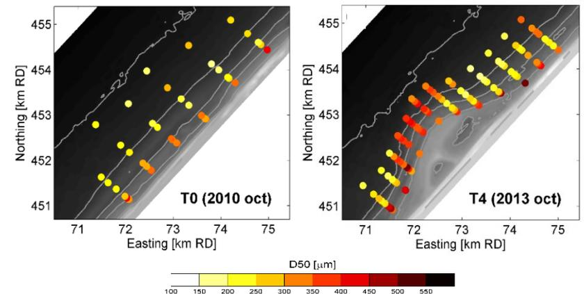
Figure 3.17 Measured median grain size ( $D_{50}$ ) for the situation before and after construction of the Sand Motor.
