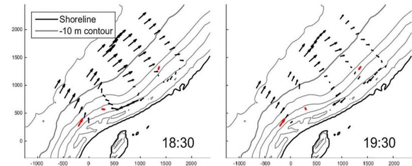
Figure 3.6 Tidal currents on the northern flank of the Sand Motor during the flood phase as recorded with a ship-mounted ADCP (Radermacher et al., 2017)
