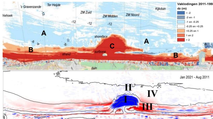
Figure 3.14 Measured bed level change in the period 1993 to 2011 and for the period 2011 to 2018. Accreting areas are shown in red, and erosion in blue.
