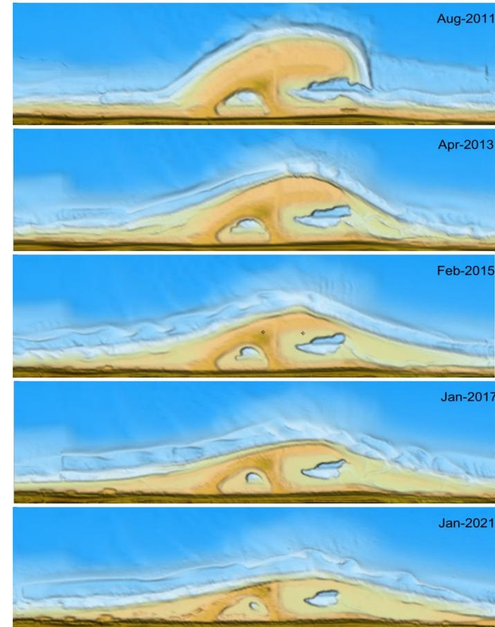
Figure 3.7 Development of the shape of the sub-tidal sand bars for the bathymetries of August 2011 till January 2021 (Huisman et al., 2021).
