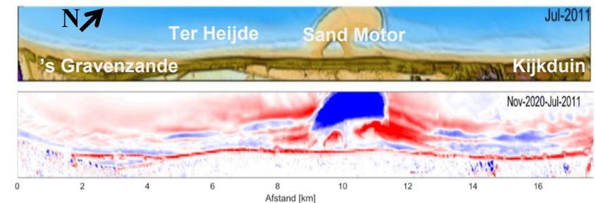
Figure 3.11 Difference in bed level of the Delfland coast between November 2020 and July 2011 (Huisman et al., 2021).
